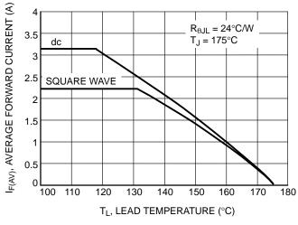
Figure 7. Current Derating, Lead
