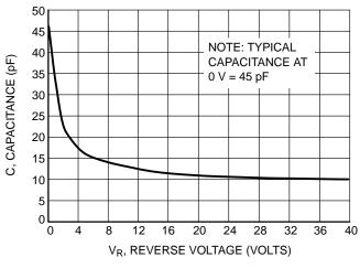
Figure 5. Typical Capacitance
