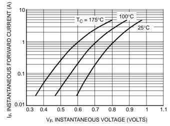
Figure 3. Typical Forward Voltage
