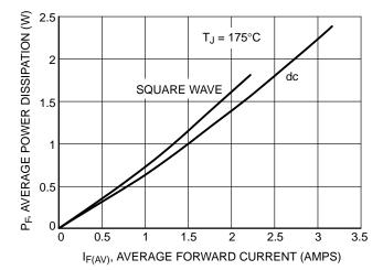
Figure 9. Power Dissipation
