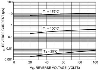
**Figure 1. Typical Reverse Current**
