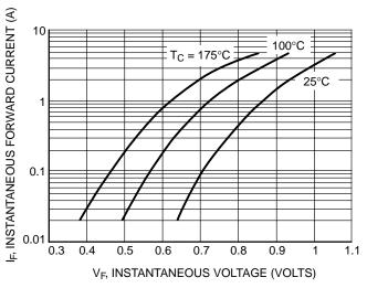
Figure 4. Maximum Forward Voltage
